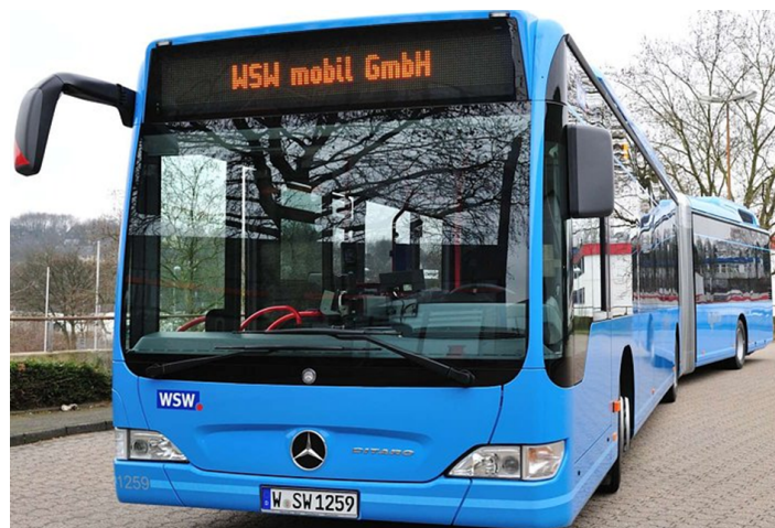
Fig. 19. Mercedes-Benz Citaro G BlueTec articulated bus with in series Hybrid drive.
