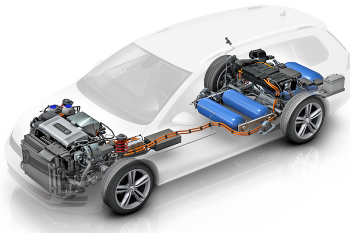
Fig. 4. Powertrain of a fuel cell electric vehicle (FCEV)
