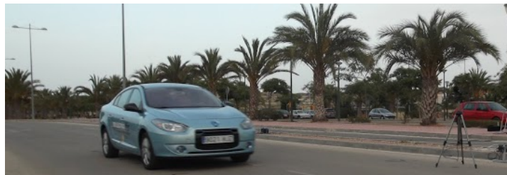
Fig. 1-Ga. Pass-by test of an Electric Vehicle
