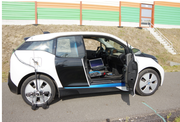
Fig.2-H. OBSIe measurement set installed on EV, BMW i3
